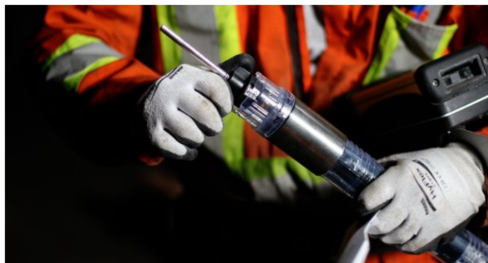
Precharging using Orica's WebGen 100 system eliminates the need for personnel to work in hazardous
