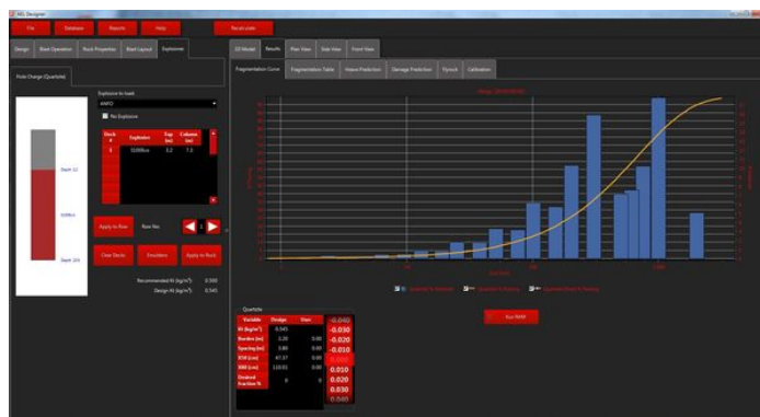
A screenshot from AEL's Designer software showing tailormaking the fragmentation of the blasted material, matching design to that required to improve shovel or haul truck or process plant efficiencies
