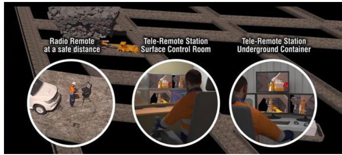
Orica has developed a fully tele-remote and mechanised Drawpoint Hang-up blasting solution with MacLean Engineering
